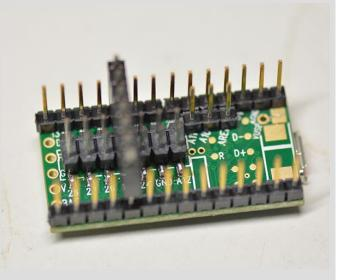
Now utilize the alignment tool yet again for the remaining 5 pins at the short end of the Teensy. You may now retire the alignment tool and call it a board header again.
