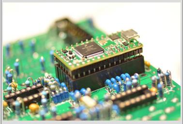
At this point, If you are not using a Panavise or other PCB clamp, remove the Teensy. You should be able to pry it out quite easily by going around it bit by bit with a screwdriver. Don't rush it and bend pins.
