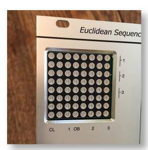
The LED matrix can be mounted without the plexiglass. The face of the matrix will be inside the panel.
