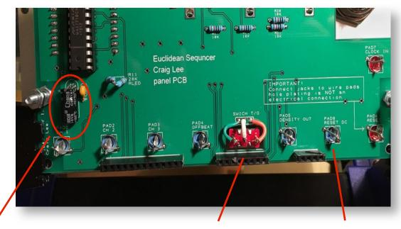
Install electrolytic capacitor laying down, this allows clearance for the PCB board above it
