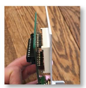
When mounting without the plexiglass use SIP sockets to mount the LED matrix.
