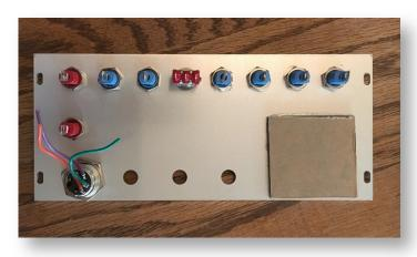
Leave space along the outer edge for mounting in an enclosure
