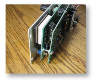
To use the plexiglass the LED matrix needs to be soldered directly to the panel PCB
